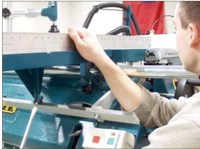
S-G Adjusting cam action of bearing to set table level.
