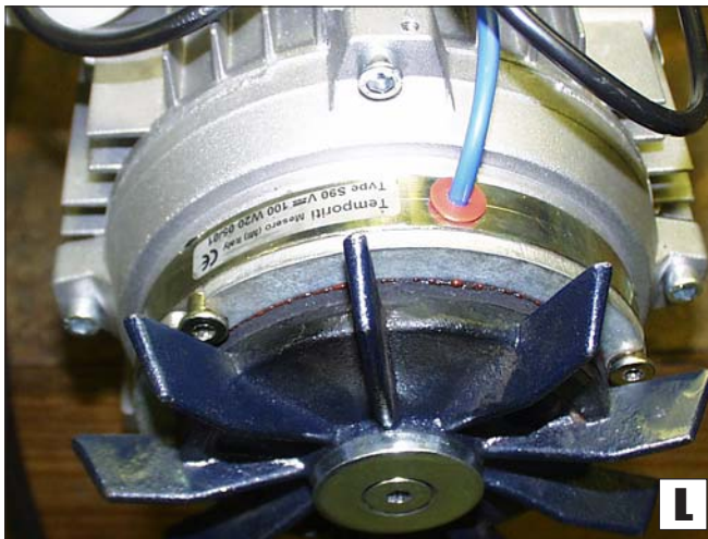
Electromagnet wire cable routed to the wiring block.
